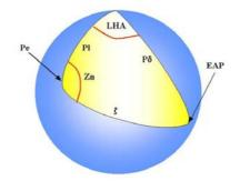
In order to apply the formulas (1) & (2) we need to convert the positions Pe and EAP in sides and angles of the navigation triangle. We will find the formulas for the navigation triangle by substitution of the converted values in the formulas (1) & (2)
