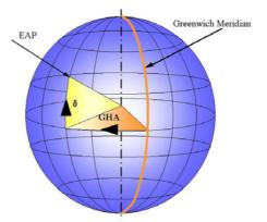
The equatorial co-ordinates system is referenced relatively to the equator and the Meridian of Greenwich. This co-ordinates system is used for describing the EAP of a celestial body. The location of the EAP on the earth's surface is fully described by two values, which are the *declination* and the *Greenwich hour angle*. Both are tabulated in the Nautical Almanac.
