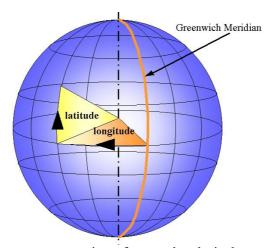
The terrestrial co-ordinates system is referenced relatively to the equator and the Meridian of Greenwich.
