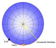
The Greenwich hour angle is the oriented angle measured along the equator from the meridian of Greenwich in western direction (clockwise when seen from above the North Pole) towards the local meridian on which the EAP is situated. Its value varies from  $0^{\circ}$  to  $360^{\circ}$  in one day. The standard abbreviation for the Greenwich hour angle is **GHA**.
